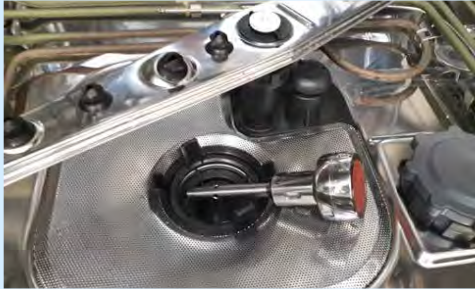
Fig. 1: The EBI 12-TC230 precision data logger being used to monitor thermal processes.
