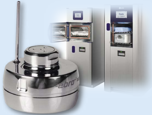
Fig. 1: Independent testing using the EBI 12-TP290 pressure-temperature data logger in the H 2 O 2 process.
