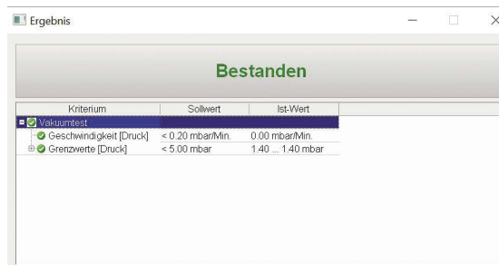
Fig. 2: Automatically generated vacuum test in accordance with E DIN EN 17180; appendix D 6.24, result with ebro Winlog.validation / Winlog.med analysis software.
