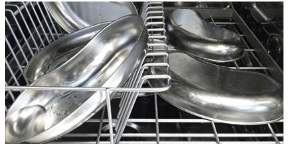
Fig. 3 Incorrect loading/kidney dishes that have toppled over.
