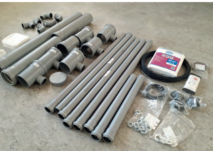
Fig. 1: Materials for a ventilation system for conference rooms.
