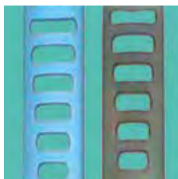
Fig. 3: Detail – titanium blades: Left blade – brand new. Right blade – cleaned by machine.
