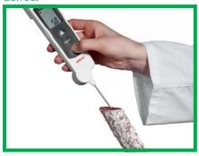
Incorrect - the probe tip may not stick out of the measured good
