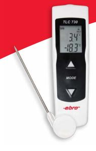
Infrared measurement devices are used to get a quick check of temperatures, for instance during incoming goods inspection. If a temperature measurement is not within tolerance, it is best to make a more accurate core temperature measurement using a penetration probe. This is especially the case when measuring through plastic or cardboard packing material. In case there is a difference between core and infrared measurements, please consider the core temperature measurement as more reliable.
