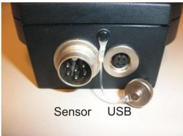
All inputs must be operated with the appropriate sensors only. Connect directly from foreign signals is not allowed.
